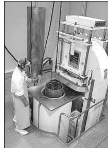
Fig 2. A batch type HPP system under operation
